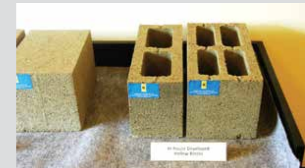
In-house Developed Hollow Blocks
