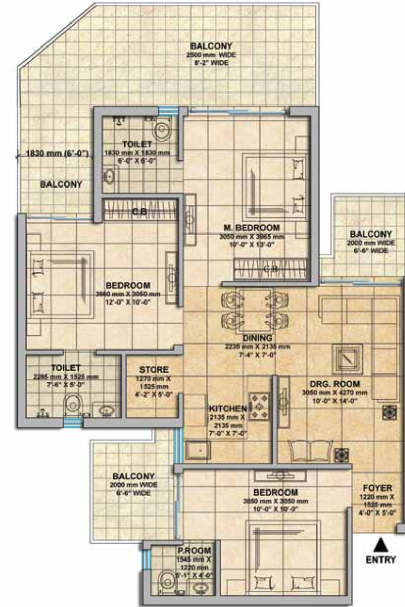
Unit Plan Type - S2 (Tower R, S) Super Built up Area - 137.10 sq.mt. / 1475.00 sq.ft. Pline Area [R.C.C. Covered Area of Flat] - 110.00 sq.mt. / 1184.00 sq.ft. 3 Bed Rooms + Drg. Room + Dining + Kitchen + Store + 2 Toilets + Powder Room + Foyer + Balconies
