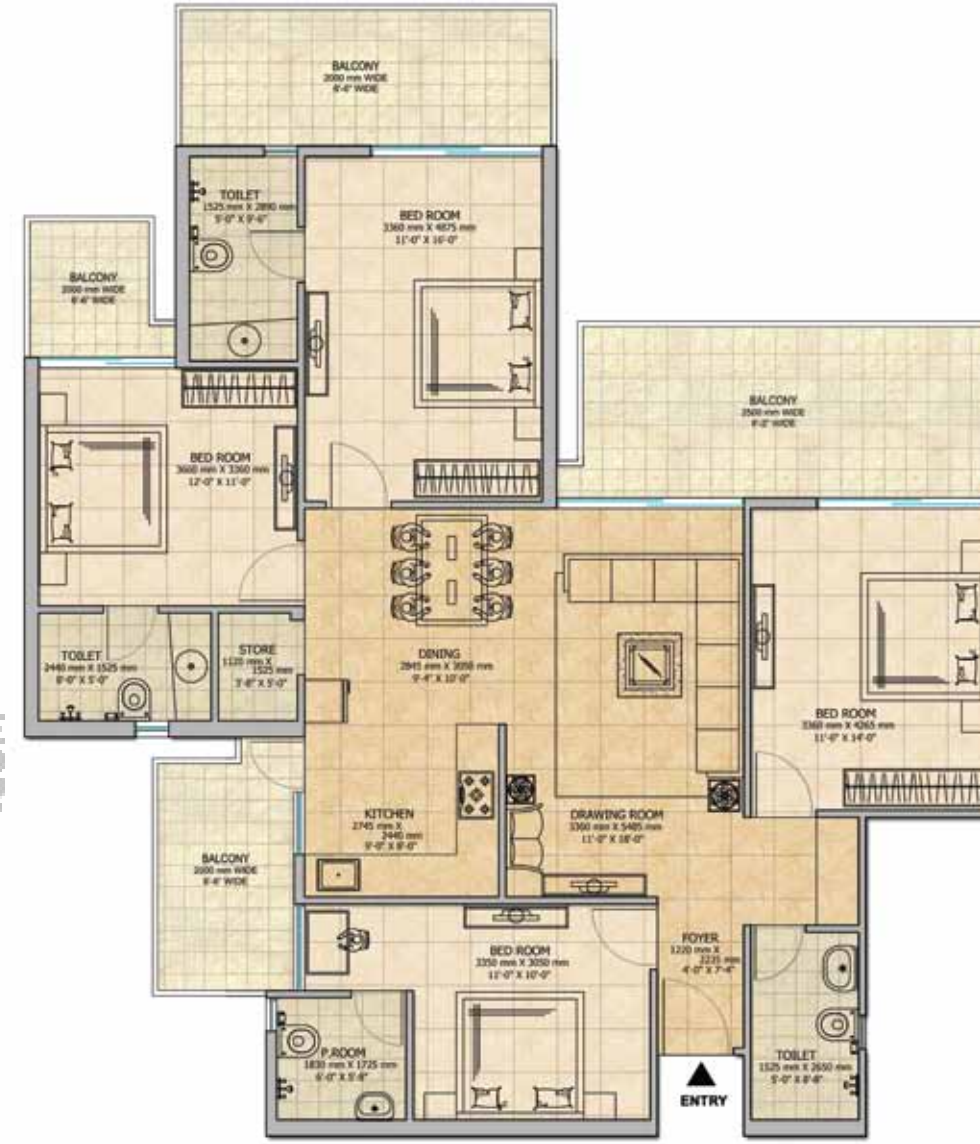
Unit Plan Type - K (Tower K) Super Built up Area - 193.24 sq.mt. / 2080.00 sq.ft. Pline Area [R.C.C. Covered Area of Flat] - 159.79 sq.mt. / 1720.00 sq.ft. 4 Bed Rooms + Drg. Room + Dining + Kitchen + 3 Toilets + Powder Room + Store + Foyer + Dress + Balconies
