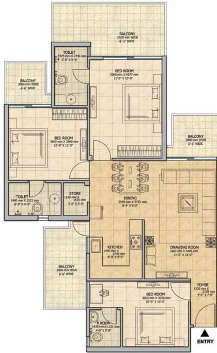
Unit Plan - Type - S-1 (Tower L) Super Built up Area - 151.43 sq.mt. / 1630.00 sq.ft. Pline Area [R.C.C. Covered Area of Flat] - 124.21 sq.mt. / 1337.00 sq.ft. 3 Bed Rooms + Drg. Room + Dining + Kitchen + 2 Toilets + Powder Room + Store + Foyer + Balconies
