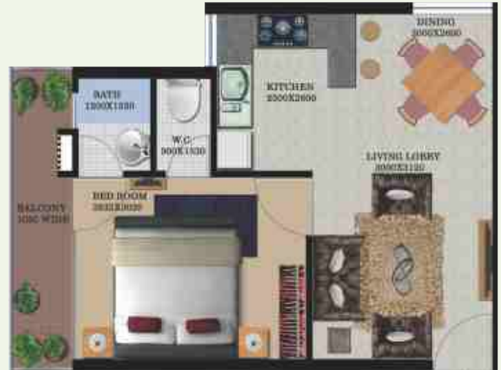
GLOBAL HEIGHTS FLOOR PLAN TYPE 5, 1BHK UNIT CARPET AREA = 392.07 SQ.FT (36.425 SQ.MTR) (Excluding Balcony)
