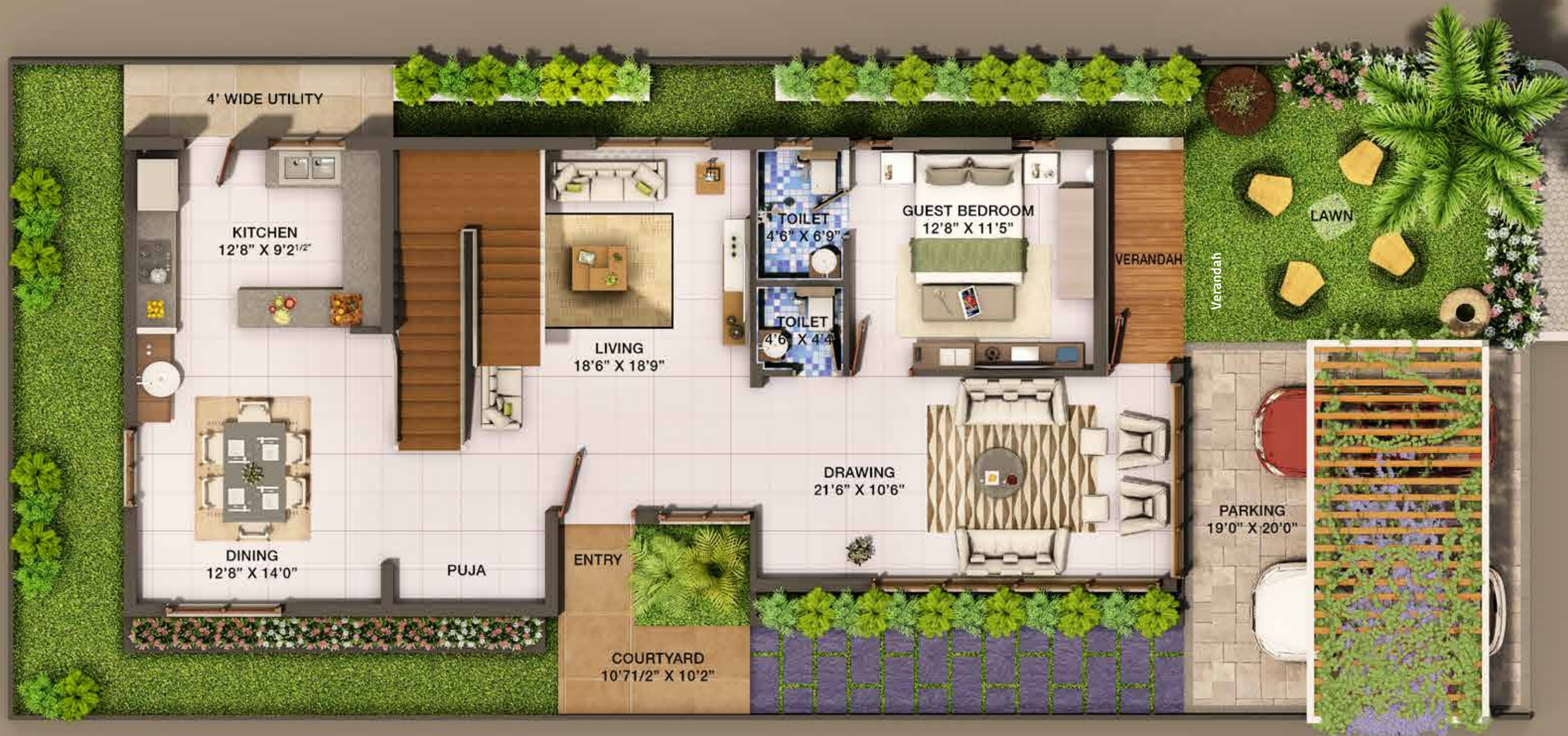
West Facing Type 'A' Ground Floor (2D Plan) Plot Area: 300 Sq.yds (34'3"X79'0") Ground Floor: 1500 sft, Parking Area: 150 sft
