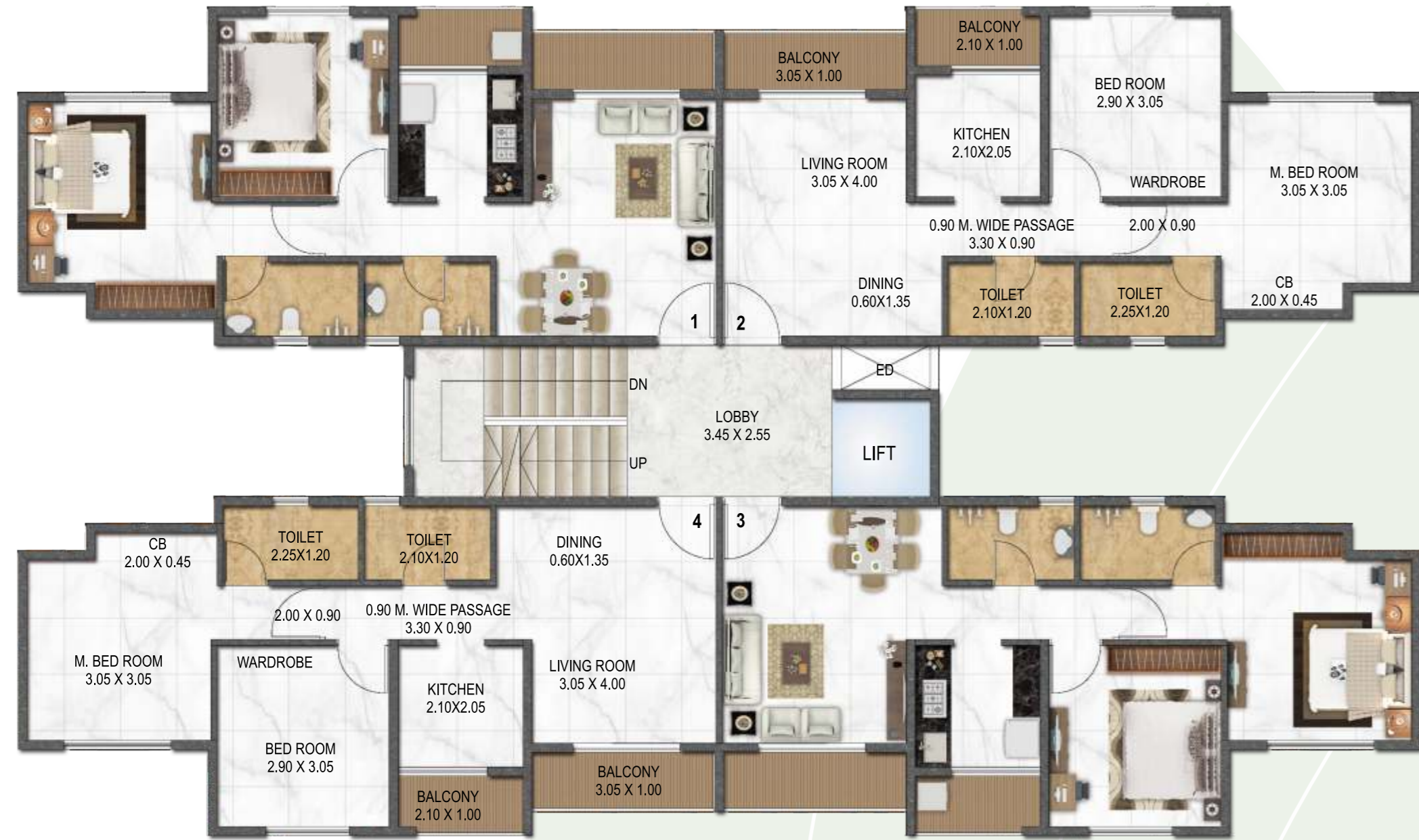
2 BHK 1 st , 2 nd , 3 rd & 4 th Typical Floor Plan (B4, B5, B6, B7, B8, B9, B10)
